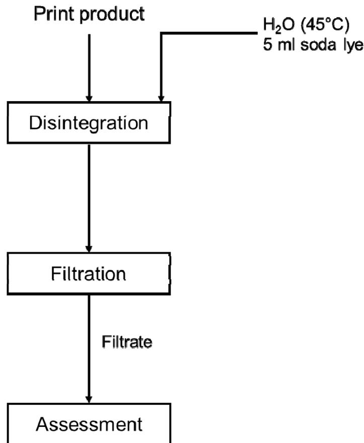
Figure 1: Flow chart of the test procedure
