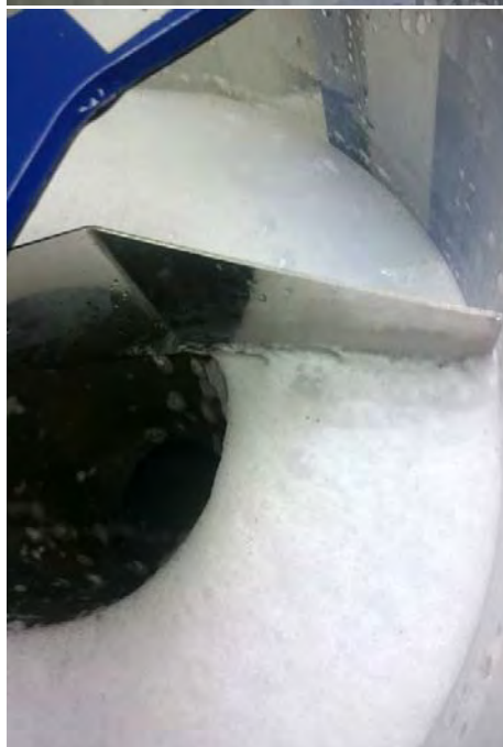
The flotation cell, in the beginning and after a few minutes of the test procedure: Air bubbling through the mixture of the sample with water and some soap carries all the ink away with the foam, leaving clean fibres
